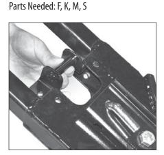
**13.** Attach four trip springs to pivot bar as shown.
