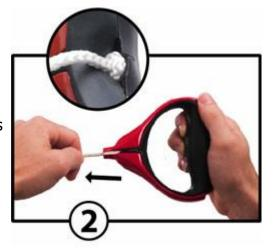
3. Remove the recoil housing from engine. Rewind starter spring counterclockwise until tight. Install rope through the eyelet, tie a knot, and pull tight. (Consult your owner's manual)
