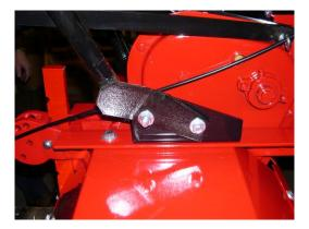
11. Attach the handlebars, tie bars and cross brace. The bolt starts to the outside of the handle and goes through (in this order) the handle bar, tie bar, cross brace. Hand tighten with a nylock nut.
