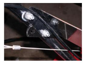
12. Attach the throttle control to the left hand handle.
