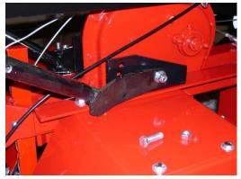
5. Attach the cross brace to the handlebars using the <u>upper</u> hole in the cross brace. <u>Be certain</u> to place two 5/16" flat washers between the handle bar and the cross brace.
