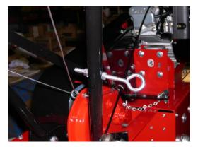
15. Check to be sure that a nut is on the end of the shift rod.
