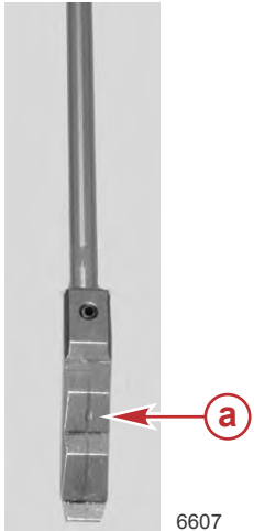
a - Shift cam ramped face
