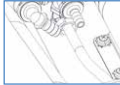
Attaches Spray Gun Hose to Pump
