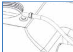
Attaches Return to Tank
