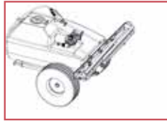
Attached Boom to Shut-Off Valve
