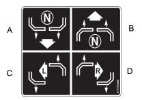
The steering levers control speed and direction. In addition, they will stop the unit.
