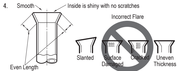
Flared Connection Dimensions / Tightening Torque.
