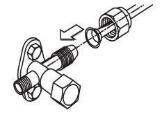
Figure 41: 18k/24k Refrigerant Pipe Connections
