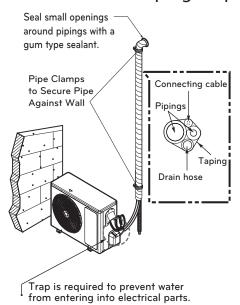
Figure 31: Cutaway of Proper Pipe and Cable Bundling
