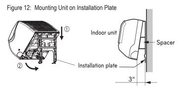
Figure 13: Mounting Unit on Installation Plate
