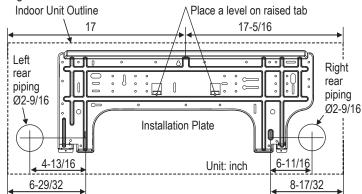
Figure 11: LAN180HYV1 / LAN240HYV1 Installation Plate Dimensions
