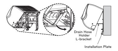
Figure 14: Chassis Cover Removal from Indoor Unit
