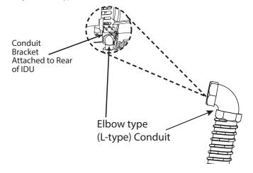
For specific bundling (taping) techniques of the Pipe and Drain Hose, see Section, "Bundling and Cutting Line" on page 36.
