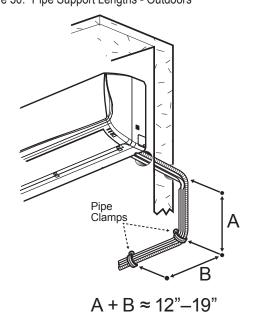
Figure 29: Installation and Piping Connection Overview
