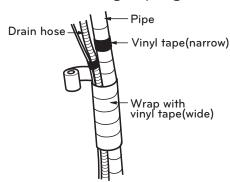
Figure 34: IDU Below ODU - Piping and Trap
