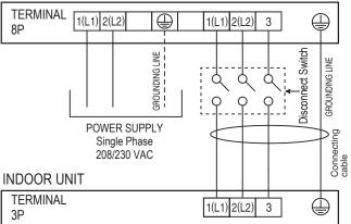
Figure 70: 18k/24k ODU to IDU Wiring
