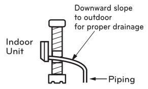
Figure 36: Correct Slope Angle for Drain Hose Incorrect Drainage Setup
