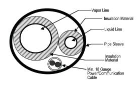
Figure 32: Bundling and Taping
