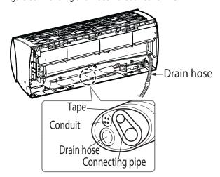
Figure 46: Piping with Insulation Material
