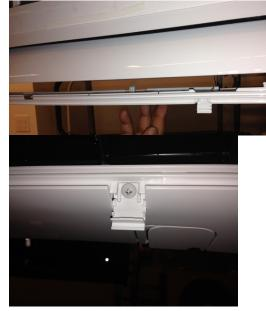
Figure 95: Remove Screws from Bottom Panel
