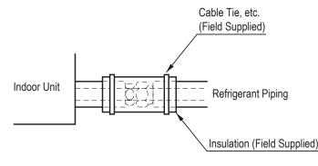
Figure 65: Typical Insulation Butt-Joint at Indoor Unit Casing.
