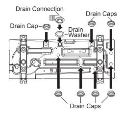
Figure 58: LSU180HSV5 Drain Component Locations. LSU180HSV5
