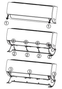
Figure 17: Removing the Bottom Cover (Appearances May Vary Depending on Indoor Unit Model).
