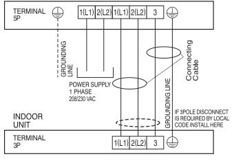
Figure 83: Typical LA240HSV3 Power / Communication System Diagram For Wiring Lengths GREATER THAN 130 Feet.
