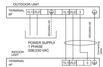
Figure 79: Typical LA180HSV5 Power / Communication System Diagram For Wiring Lengths Up to 130 Feet.
