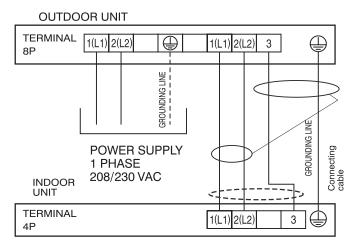
Figure 84: Schematic of a Single Zone System When the Wiring is GREATER THAN 130 Feet.
