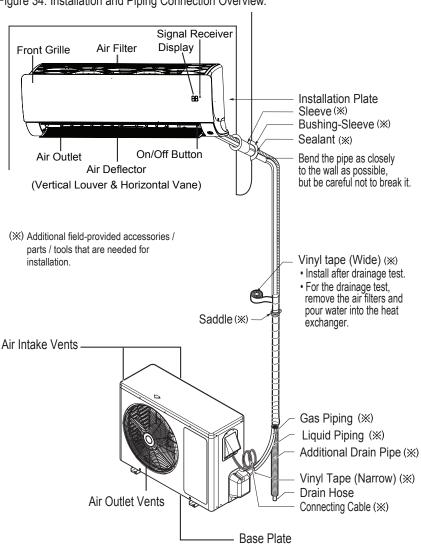
Figure 34: Installation and Piping Connection Overview.
