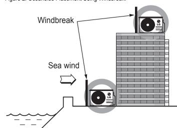
Figure 3: Placement Using Building as Shield.
