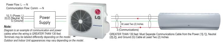
Figure 82: Typical LA180HSV5 Power / Communication System Diagram For Wiring Lengths GREATER THAN 130 Feet.
