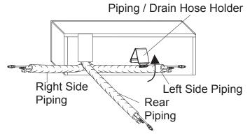
Figure 43: Bending Piping at Rear of Indoor Unit.
