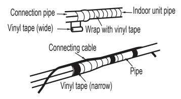
Figure 63: Cutaway of Proper Pipe and Cable Bundling.
