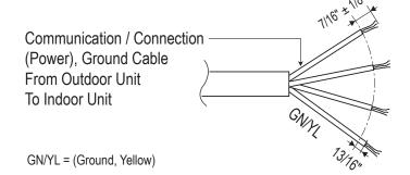
Figure 77: Single Zone Outdoor Unit to Indoor Unit Wiring and Communications Cable Diagram For Wiring Lengths GREATER THAN 130 Feet.
