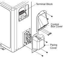
Figure 38: LSU090-120HSV5 Piping Connections.
