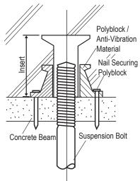
Figure 7: Close up of Bolt Attachment.
