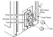
Figure 106: Triple Leak / Pressure Test Diagram.
