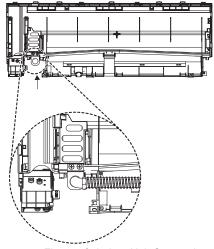
Figure 50: Indoor Unit Connection.
