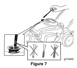
2. Remove the dipstick and check the oil level (Figure 7). If the oil level is below the Add mark on the dipstick, **slowly** pour oil into the oil fill tube to raise the oil level to the Full mark on the dipstick. Do not overfill. (Max. fill: 22 oz. (0.65 l), type: 10W-30 or SAE 30 detergent oil with an API service classification of SJ or higher.)
