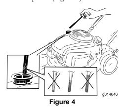
Slowly pour oil into the oil fill tube until the oil level reaches the Full line on the dipstick (Figure 4).
