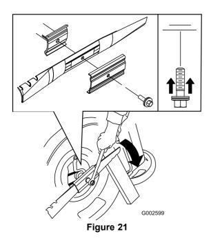
**Important**: Position the curved ends of the blade to point toward the mower housing.
