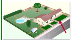
The secondary area is a part of the yard separated from the primary area but connected to it with the going in and out of cable.
