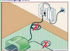
Pay attention to the sprinkler system! It is necessary to understand where the sprinklers are and place the recharging base in a safe part of the yard far from the sprinklers that might wet the back of the robot. The concept is that water must not enter the recharging base.
