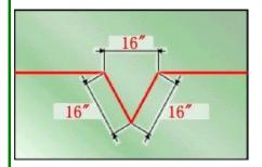
The rapid return or "Arrow", is a perimeter cable symbol recognized by the robot in order to come back quickly to the recharging base. There are many advantages:
