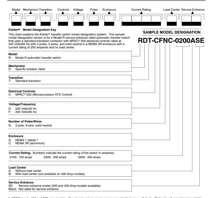
\* NEMA 1 only: 100 and 200 amp models without load centers can be recess-mounted between wall studs. Optional wall-mount bezel available. The NEMA 1 enclosure for 400 amp models is aluminum.
