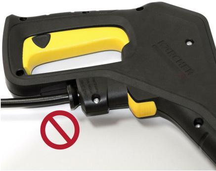
The entire hose connection should be seated inside the spray gun. If you can still see the hose connector, the hose is not properly attached and will result in leaking, as well as weak pressure when using the power washer.
