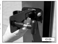
8. Block the wheels to prevent the base unit from moving. Carefully lower the rail assembly to a horizontal position. Securely tighten the nuts holding the base unit to the rail assembly (Step 6) and the nuts holding the rail rest assembly (Step 7).
