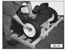
3. Before removing the base unit from the pallet, remove the tongue and front leg assembly and install it to the base unit using four 1/2-13 x 1-1/2 inch long hex head bolts, lockwashers, and nuts. Tighten the nuts securely. Roll the tongue/base unit off the pallet. Lower the front leg and lock it into position.
