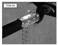
Place a customer supplied lock or lock pin into the latch assembly of the hitch coupler.
