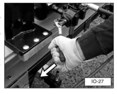
d. Once the wedge reaches its full forward travel, pull back on the control lever to the full retract position. The ram of the cylinder will automatically retract into the cylinder. It is not necessary to hold the control lever as the cylinder retracts. Stop the wedge if the log sticks (see caution below). When the cylinder is fully retracted, the control valve will automatically shift to a neutral position.
