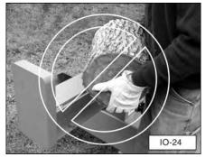
**b**. Only using your hand, push the control lever forward (towards the log). If the log moves, before it is contacted by the splitting wedge, release the control lever and then reposition the log. Operate the log splitter only when standing in the safe operating area. shown in the picture.
