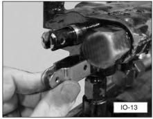
12. Install the valve handle onto the valve link using a 1/4 x 3/4 inch long clevis pin. Secure the clevis pin with a cotter pin (bend the ends of the cotter pin to make it secure).
