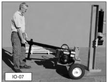
**6**. Bolt the base unit to the rail assembly using two 1/2-13 x 1-1/2 inch long hex head bolts, lockwashers, and nuts, as shown. Hand tighten the nuts.
