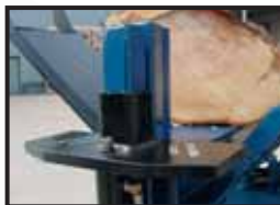
Hydraulic 4-way wedge adjusts easily to desired height with push or pull of valve lever.
