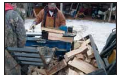
With tow hitch / mobile stabilizing jack assembly removed, a wheel loader bucket conveniently fits under the splitting wedge to assist in gathering of split logs.
