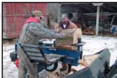
With tow hitch / mobile stabilizing jack assembly removed, a wheel loader bucket conveniently fits under the splitting wedge to assist in gathering of split logs.
