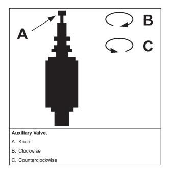
Select constant speed control if the unit restarts in less than 10 minute intervals or runs more than 40 minutes per hour. Turn the knob fully counterclockwise to run the unit continually.
