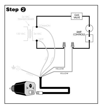
Cut-off the connectors and strip the ends of the two yellow wires of the Model 1100 harness. Break into the burner circuit between the *hot* side of the transformer (R) and other limit controls. Connect either YELLOW wire to the *hot* side. Connect the other YELLOW wire in series with other limit controls. Important: The switch contacts of the low water cutoff (yellow wires) must be wired in series with all other limit and operating controls (as shown above).
