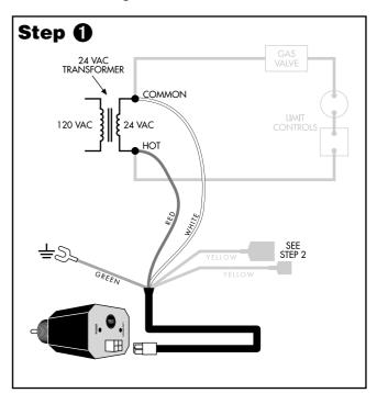
Connect RED wire to *hot* side of 24 Volt boiler transformer (R). Connect WHITE wire to common side of 24 Volt boiler transformer (C). Connect the GREEN wire to any suitable, unpainted ground screw. **Note:** for operation of the control, the green wire must be connected to a ground source electrically common with boiler ground.
