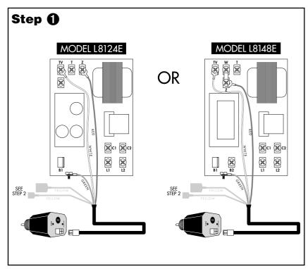
Connect the WHITE wire to **TV** and the RED wire to **Z**. Connect the GREEN wire to the ground screw on the bottom of the aquastat or any other suitable, unpainted ground screw. **Note:** for operation of the control, the green wire must be connected to a ground source electrically common with boiler ground.
