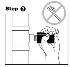
Hand tighten the control into boiler tapping or pipe tee. Be careful not to cross thread. **Note:** Do not use a wrench. Hand tighten only.
