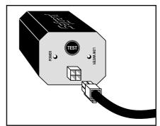
Plug wire harness into connector on face of control.
