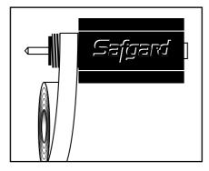
Apply Teflon® tape to the threads of the Model 1100. Do not use pipe dope or other pipe sealants.
