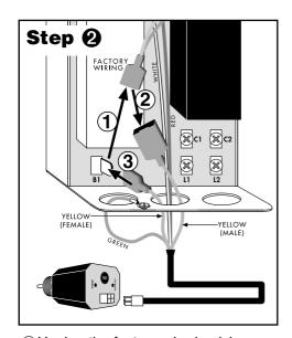
① Unplug the factory-wired quick connect from terminal **B1** and ② plug into YELLOW wire with *male* connector.
