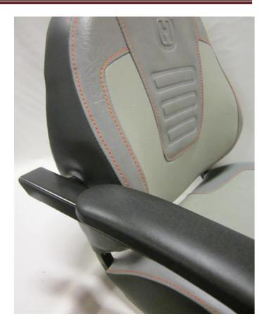
9) Press arm pin approximately 1 ½" into bracket. Wiggle arm frame up and down until it will rotate 180 degrees and land in its home position.
