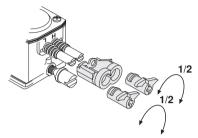
When your chain saw is equipped with a carburettor that features movement limiters, the carburettor should be adjusted according to the instructions under the heading Carburettor with movement limiters.
