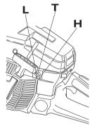
The T-screw regulates the throttle setting at idle speed. If the T-screw is turned clockwise this gives a higher idle speed; turning it anti-clockwise gives a lower idle speed.
