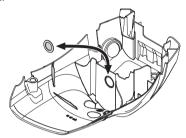
For running the machine in cold weather or powder snow, a special cover is available, which is mounted on the starter housing. This reduces the intake of cold air and prevents large amounts of snow from being sucked in.
