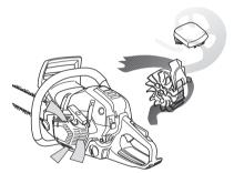
IMPORTANT! In order to maintain operation of the centrifugal cleaning system it must be regularly maintained. Clean the air intake to the starter, the fins on the flywheel, the space around the flywheel, inlet pipe and carburettor compartment.
