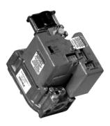
The TRADELINE® SV9541 SmartValve System Controls combine gas flow control and electronic intermittent pilot sequencing functions into a single unit. The Q3450 or Q3480 Pilot hardware supplies the low voltage igniter, flame sensor and pilot burner. These ignition system controls provide all gas ignition safety
