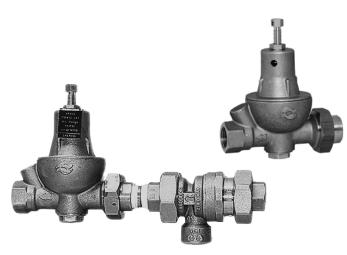
Pressure regulating valve for automatic control of boiler feed water and other pressure reducing applications. Especially constructed for expansion tank mounting.
