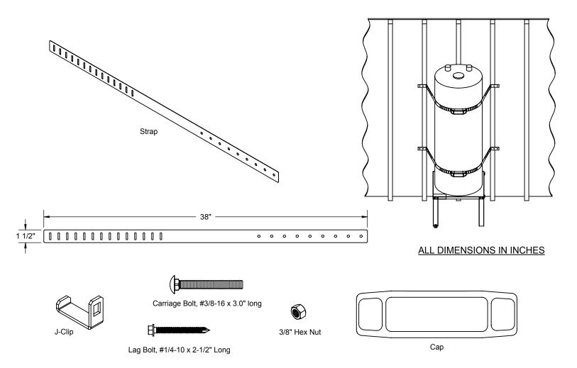
The QUICK STRAP® #QS-50-D is a seismic/earthquake support system for water heaters up to 80 U.S. gallons in size. The system includes: (4) Straps, (4) J-Clips, (4) Lag Bolts, (2) 3/8" Carriage Bolts, (2) Caps and (2) 3/8" Hex Nuts. The Quick Link® system allows for full adjustment from the front side of the water heater.
