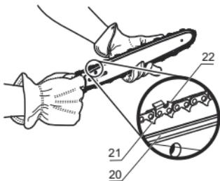
7. Ensure the chain is put on in the correct direction (do not assemble with the cutters backwards).
