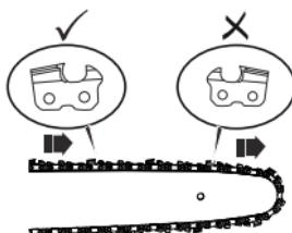
8. Put the chain in position and make sure that the loop is behind the guide bar.
