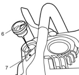
4. Put the oil into the oil tank. Be careful not to let the oil spill from the opening. Wipe off any excess oil.
