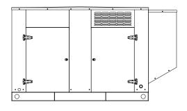
"LEVEL 2" HOUSED GEN-SET Full aluminum weather protection and superior sound attenuation for specific low noise applications. Critical grade muffler is standard.
