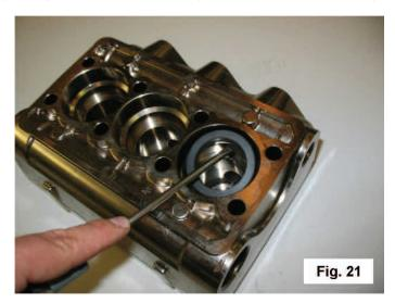
Pay attention to the order of seal pack disassembly as indicated in fig. 23 composed of:
