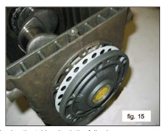
Once the type and number of shims have been determined using the table, check the following: assemble the shim pack on the indicator side cover centering (fig. 15). Secure the cover to the casing, following the procedure in part 2.1.2 and tighten the screws to their recommended torque. Check that the shaft rotation stall torque is between 3-4.3 ft.lbs.(4-6 Nm).
