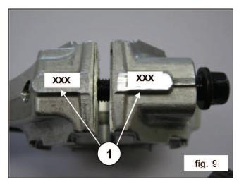
Fasten the caps to their respective con-rod shanks by means of M8x1x48 screws (fig. 10) lubricating both the underhead and the threaded shank. Proceeding in two different stages.
