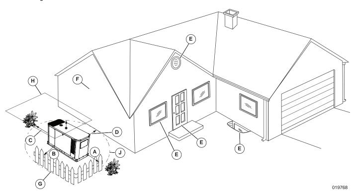
Figure 3-2. Generator Distance Requirements
