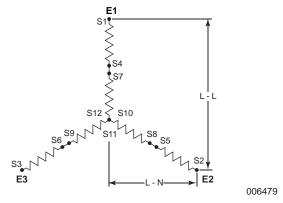
Figure 10-3. Stator Power Winding Connections—3-Phase, 480/277 V (12 Lead)
