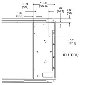
Figure 3-4. Installation Drawing Stub-Up Detail (Typical)
