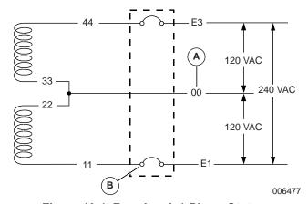
Figure 10-1. Four-Lead, 1-Phase Stator
