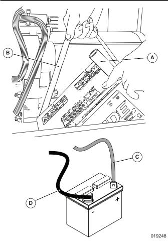
Figure 5-8. Battery Cable Connections
