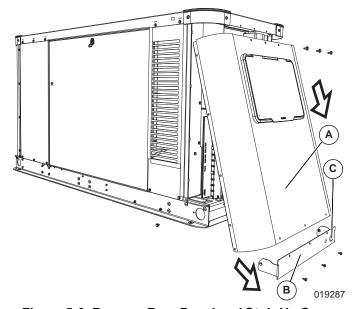
Figure 5-6. Remove Rear Panel and Stub-Up Cover
