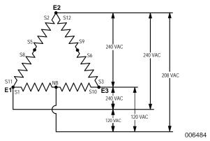
Figure 10-4. Stator Power Winding Connections—3-Phase, 240/120 V (12 Lead)
