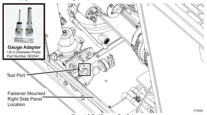
Figure 4-5. Fuel Pressure Test Point
