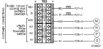
Figure 5-4. TB2 Control Wiring Connections - 3-Phase
