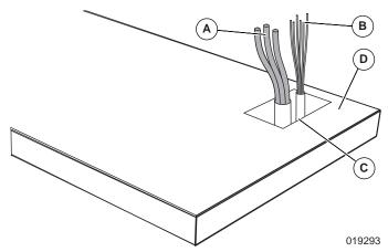
Figure 5-5. Typical Load Leads and Control Wiring in Stub-Up
