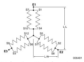
Figure 10-2. Stator Power Winding Connections—3-Phase, 208/120 V (12 Lead)
