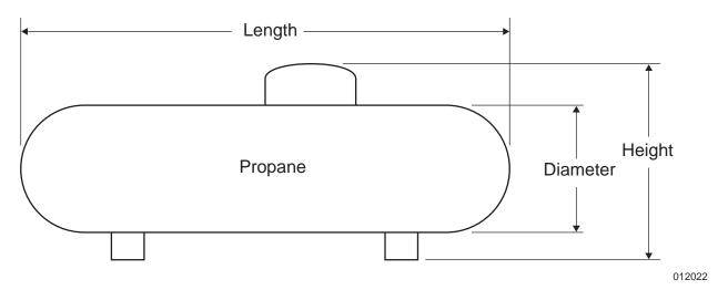
Figure 4-3. Typical Propane Tank Dimensions
