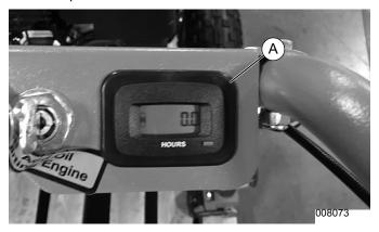
Figure 2-21. Maintenance Meter Installation
