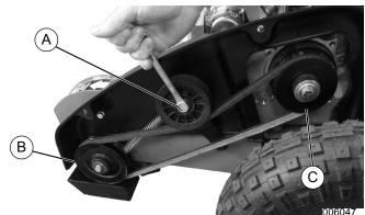
Figure 4-8. Belt Guard Bolts and Locknuts
