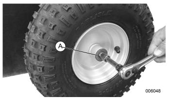
Figure 4-17. Replacing the Wheels
