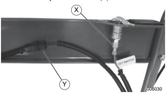
Figure 2-16. Key Switch Connector
