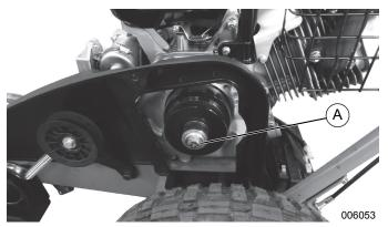
Figure 4-9. Replacing Clutch
