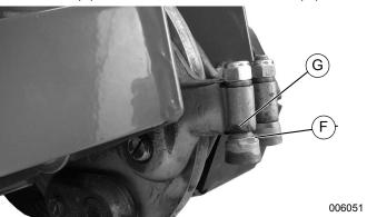
Figure 4-12. Rotating Cutting Teeth
