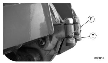
Figure 4-14. Replacing Cutting Teeth
