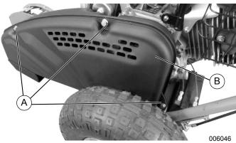
Figure 4-7. Belt Guard Bolts and Locknuts
