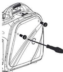
Figure 4-3. Remove Side Cover
