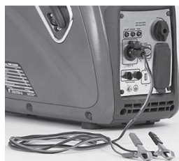
Figure 3-4. Battery Charger Input Jack
