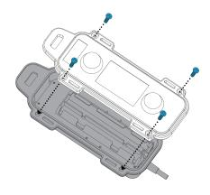
▲ WARNING: EXPLOSION HAZARD - BATTERIES MUST ONLY BE CHANGED IN AN AREA FREE OF IGNITEABLE CONCENTRATIONS. **AVERTISSEMENT:** RISQUE D'EXPLOSION - LES BATTERIES NE DOIVENT ÊTRE REMPLACÉES QUE DANS UN EMPLACEMENT EXEMPT DE CONCENTRATIONS INFLAMMABLES.
