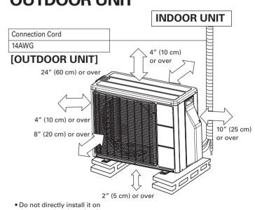
the ground, otherwise it will cause failure
