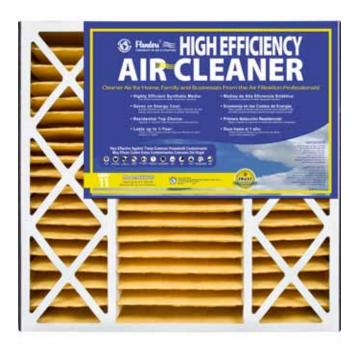
The High Efficiency Air Cleaner MERV 11 consist of efficient, high quality synthetic media. The Deep V-Pleats allow 5x more media than standard filters, providing greater surface area. This reduces airflow restriction for less energy consumption, increasing the effective life of the filter.
