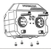
The Parallel Kit can be mounted using 4 X M6-1.0 screws(not included) before connecting to the inverter.
