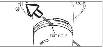
FIGURE 15: Pull old mower line out through exit hole
