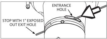
FIGURE 16: Insert new mower line into entrance hole
