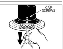
FIGURE 11: Threading Mower Line Through Center F Hold.
