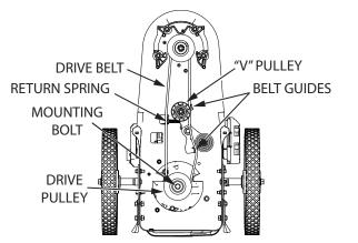
FIGURE 21: Routing The Drive Belt
