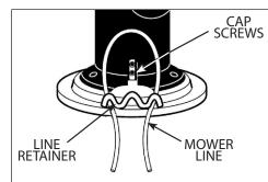
FIGURE 10: Threading The New Mower Line.
