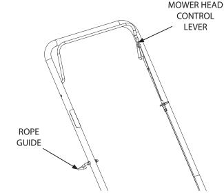
FIGURE 5: Using The Mower Head Drive Lever.
