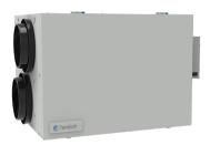
Suitable for very large residential or small commercial applications, the compact SER 260D comes with access panels on both sides of the unit for installation versatility. The SER 260D unit brings a continuous supply of fresh air into a home while exhausting an equal amount of contaminated air. The enthalpic core at the center of the unit transfers heat and moisture from the incoming air to the outgoing air that was cooled and dried by the building's air conditioner.
