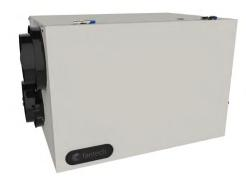
Fantech's, SER 150 is an Energy Recovery Ventilator designed for higher static pressure applications. The unit brings a continuous supply of fresh air into a home while exhausting an equal amount of contaminated air. The energy recovery core at the center of the unit transfers heat and moisture from incoming air to the outgoing air that was cooled and dried by the building's air conditioner.
