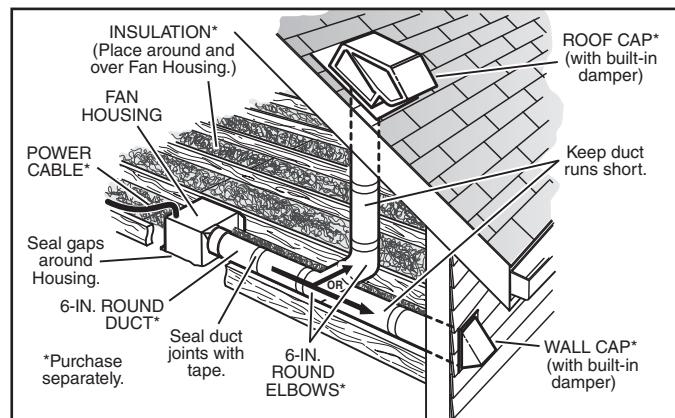
The ducting from this fan to the outside of the building has a strong effect on the air flow, noise and energy use of the fan. Use the shortest, straightest duct routing possible for best performance, and avoid installing the fan with smaller ducts than recommended. Insulation around the ducts can reduce energy loss and inhibit mold growth. Fans installed with existing ducts may not achieve their rated airflow.
