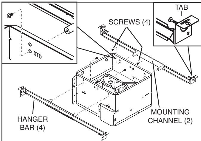
Attach the **MOUNTING CHANNELS** to the housing using the **SCREWS** supplied. Make sure **TABS** face "up" as shown. Use the set of channel mounting holes (marked "STD") to mount the housing flush with the bottom of the drywall. Use the other set of holes (not marked) to mount the housing flush with the top of the drywall.
