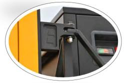
Patented swing arm mount for quick and easy maintenance, simply take out the pin and swing the dryer to the side accessing the door panel. Making the unit more compact taking up less space!
