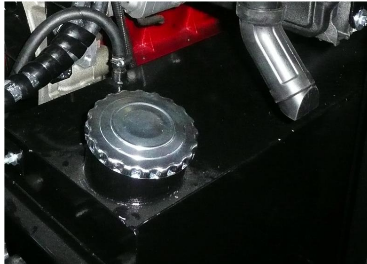
Figure 10.1-2 Gas oil tank for Diesel engine
