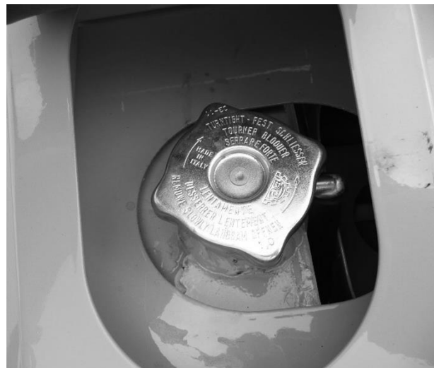
Figure 10.1-3 Checking the radiator cooling liquid
