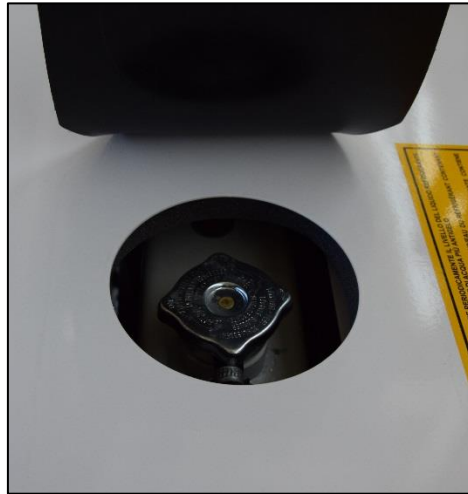
Figure 13.4-3 Checking the coolant radiator
