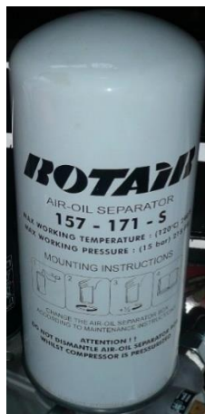
Figure 13.4-7 Oil separator filter
