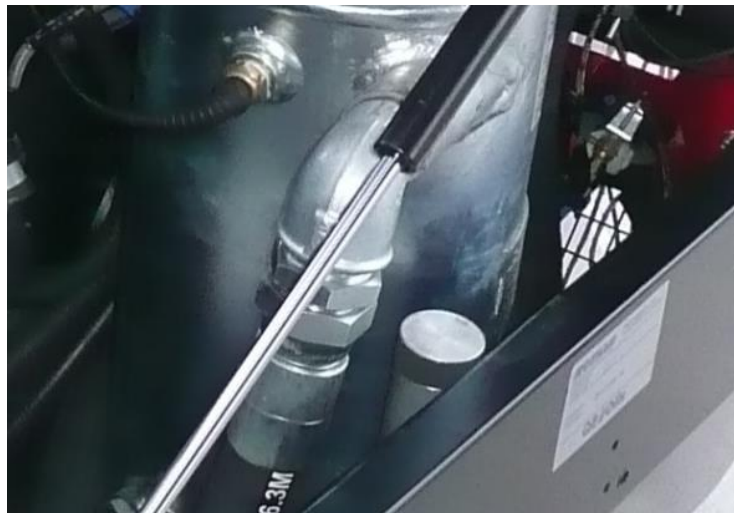
Figure 10.1-1 Checking the oil level in the compressor
