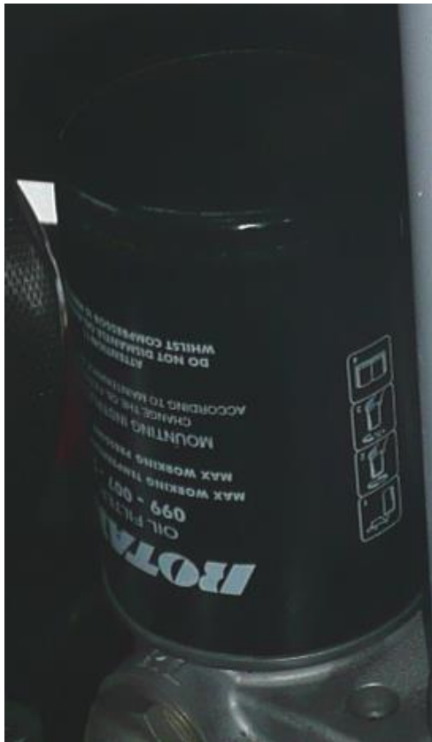
Figure 13.4-6 Compressor oil filter
