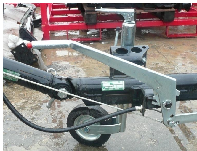
Figure 6.4-2 Lever of the manual park brake with release red push-button
