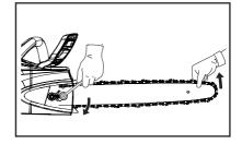
Pull the chain around the bar by hand. Loosen the tension adjuster if you feel tight spots while rotating chain on the bar by hand.
