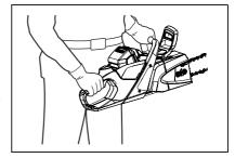
Squeeze the trigger switch to increase motor speed to maximum rpm and start the cut. If the chain is properly sharpened, the cutting should be relatively effortless. It is not necessary to press down hard to make the saw cut. Pushing the saw too hard will slow the motor speed and cutting will actually be more difficult.
