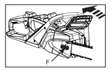
Tighten sprocket cover nuts with the bar nose held up and under tension.
