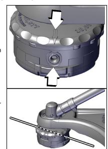
4. Hold trimmer head while turning knob clockwise to wind line onto spool until about 13 cm (5 in.) of each line remains exposed.
