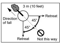
Begin the cut on the side to which the tree is to fall. Cut a notch about 1/3 of the way into the tree. The position of this notch is important since the tree will try to fall "into" the notch. The felling cut is made on the side opposite the notch and at a level about 5 cm (2 in.) above the bottom of the notch. Do not try to cut through to the notch with the felling cut. The remaining wood between the notch cut and felling
