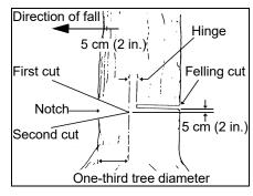
cut about 5 cm (2 in.) will act as a hinge when the tree falls, guiding it in the desired direction. When the tree starts to fall, kill the engine, place the saw on the ground and make your retreat guickly.
