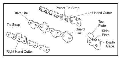
Important points for proper maintenance of saw chain:
