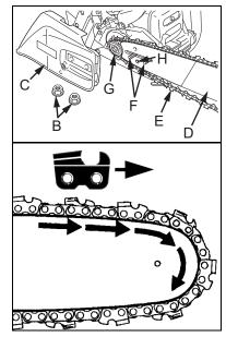
7. Adjust saw chain tension, as instructed in "Adjustment, Chain Tension".
