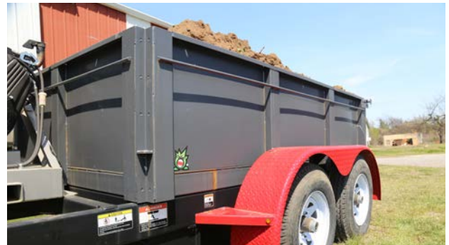
Removable top walls convert the container for hauling
