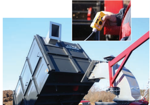
Hydraulic lift, 50° dump angle
