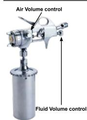
Air and fluid volume controls: These two controls are used in conjunction with each other to accurately adjust air/fluid (Paint) ratio and will vary for different paints. Changing one control affects the other so alternating back and forth between them to fine tune your adjustment will yield optimum results
