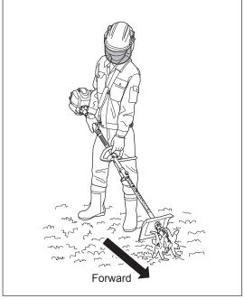
The blade will rotate in the direction of forward movement.
