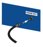
**Step 3:** Connect the included propane line to the propane tank.
