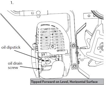
Be sure the engine is located on a level surface before checking or refilling oil. Proper position for checking oil level or refilling oil is face down, with the gas tank of the Tiller/Cultivator down on a horizontal surface (*Figure 4*).
