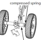
locking metal sleeve (**LOCKED** position) locking metal sleeve (**UNLOCKED** position)
